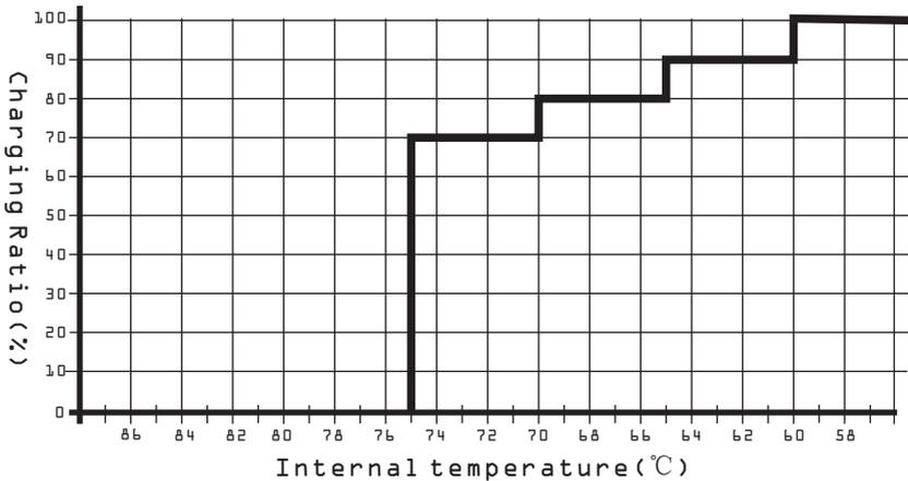
X-axis is the internal temperature, Y-axis is the charging ratio.
